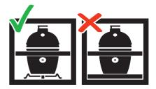
A stainless steel table nest should always be used to create an air gap between the Kamado and the outdoor kitchen. Do not place the Kamado directly on the surface of the outdoor kitchen.
